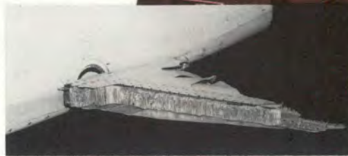
This is all that remained of the left horizontal tail of the T-38.
