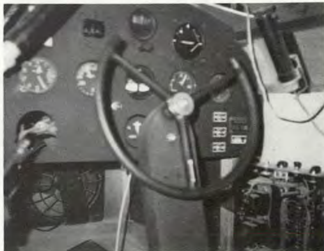
The Link Trainer, Model C-3, was first delivered to the Army Air Service in 1934 and remained in use through WWII. Pilots in IPIS received instrument procedures training in this model trainer. Do you suppose they made the exterior resemble an airplane to help the pilot pretend he was flying?
