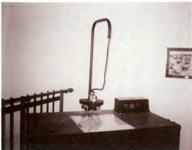
While the pilot flew the trainer through various climbs, turns, and descents, his course was traced in ink on the map on the table. After the flight, the instructor and the pilot could review the lines on the map to determine what the pilot had done.
