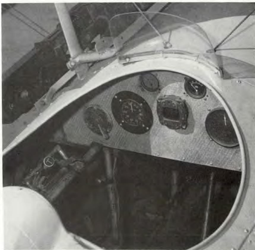
Early aircraft were fitted with a minimum of instruments. The turn and bank indicator either wasn't included or was mounted in an out-of-the-way location that made it almost useless.
