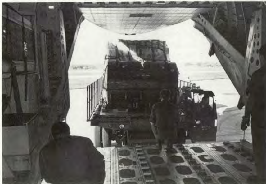
The C-141 can airlift combat forces, equipment, and supplies and deliver them on the ground or by airdrop. This cargo capacity was increased by 30 percent when all C-141A models were modified to lengthen the fuselage.
