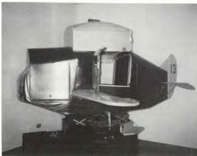
The Link Trainer, Model C-3, was first delivered to the Army Air Service in 1934 and remained in use through WWII. Pilots in IPIS received instrument procedures training in this model trainer. Do you suppose they made the exterior resemble an airplane to help the pilot pretend he was flying?
